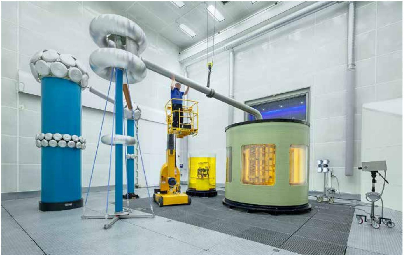
MR Test Center – High-tech laboratory for on-load tap-changers
